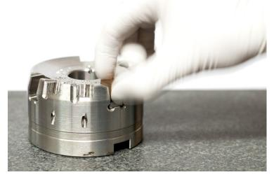
2. Once seated, using your thumb or finger, push down on the top of the wiper insert to keep it from moving while tightening the screw. Place the screw into the wiper and torque it to the recommended spec for that wiper and screw.
