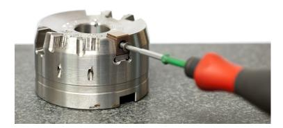
3. Remove wiper inserts from cutter body and clean them. **DO NOT** remove wiper shims from pockets.
