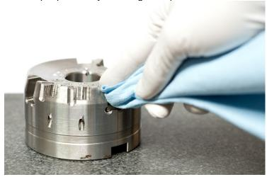
5. Check wiper pockets for wear or any nicks/burrs that need to be removed.
