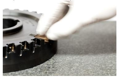
2. Place the screw into the wiper and torque it to the recommended spec for that wiper and screw.
