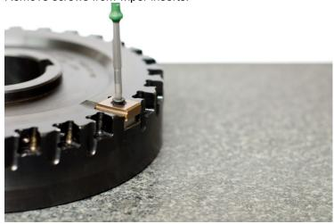
3. Remove wiper inserts from cutter body and clean them. **DO NOT** remove wiper shims from pockets.
