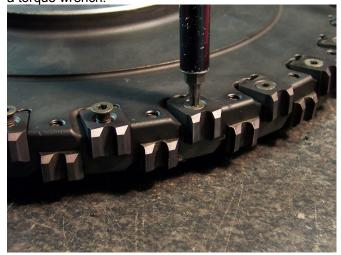
5. After all inserts have been installed in the pockets, use a torque wrench to make sure that all screws are tightened to the proper torque that is recommended for that insert and screw.
