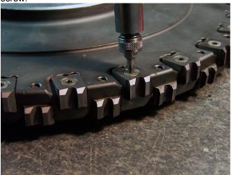
Note: Insert pocket is error proofed. The screw will not go in if the insert is in wrong.
