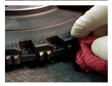
6. <u>Check inserts pockets for wear or any nicks/burrs that need to be removed.</u>
