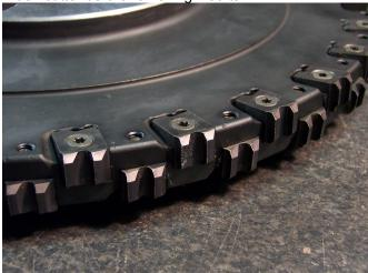
2. Remove all screws from cutter body.
