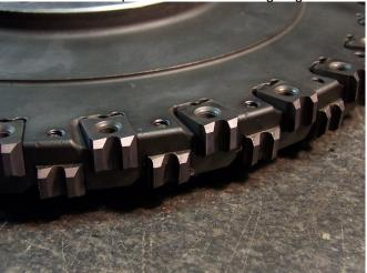
2. Slide insert back and forth in the pocket to insure that it is seated properly.
