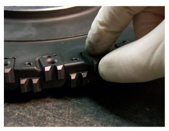
3. Once seated, hold insert into the back of the pocket by pushing with thumb or finger on cutting edge of insert.
